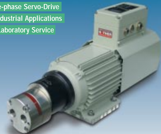
Three-phase motor (IP 55) for industrial applications and laboratory service, controlled via frequency converter, n = 10 - 3,000 rpm, external control capability, 1 x 230 V, 50 Hz
