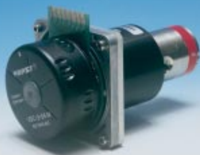
Brushless DC motor (IP 00) of compact design, ideal for integration into miniature units, n = 350 - 3,500 rpm, external control capability, 0 - 10 V, supply voltage 24 V, favorable price/performance ratio
