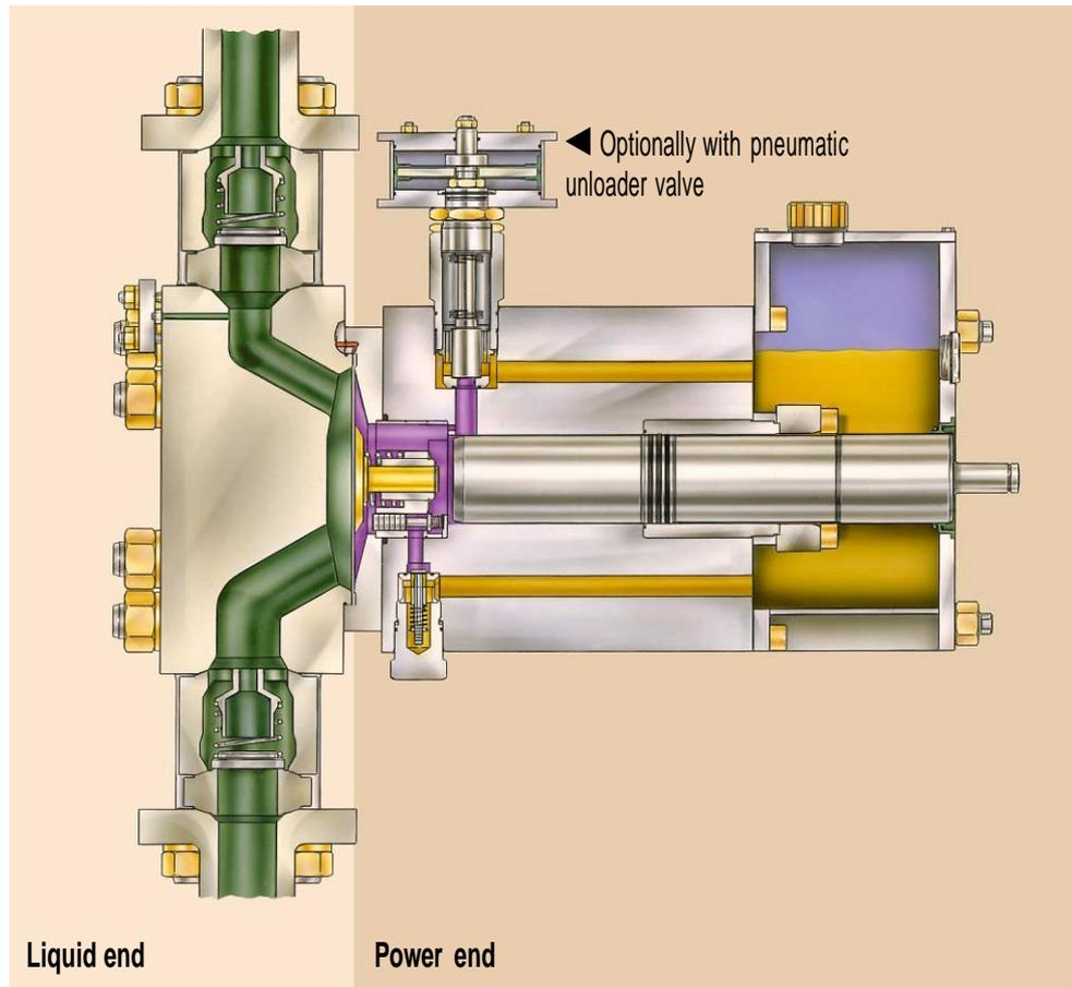
If a single diaphragm begins to leak, the rupture signal is operational thus allowing sufficient time to normally shut down the process and/or to bring a stand-by pump into operation.
