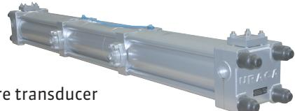
The oil hydraulically driven pressure transducer is an alternative of the conventional plunger pumps to be used on sewer cleaning vehicles. It is driven by a variable displacement axial piston pump in closed circuit. The oil tank has an integral oil cooler passed by the medium. For cleaning purpose its covers can easily be removed.
