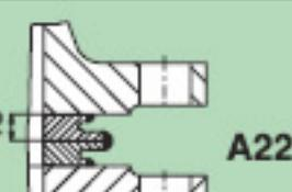
A22 | a) An additional intermittent weld for further fastening<br>b) If susceptible to corrosion | a) Standard procedure<br>b) Additional fastening Befestigungshilfe. through intermittent weldments | hardly possible<br>max.. $\Delta r \sim 0,1$ mm                                            | Use cut-off disc.<br>Material loss 2-3 mm each.<br><br>Can be rewelded up to 5 times |
