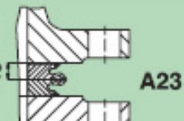
A23 | a) An additional intermittent weld for further fastening<br>b) If susceptible to corrosion | a) Standard procedure<br>b) Additional fastening through intermittent weldments                    | Effect is small because of the small hollow lip dimensions.<br>max. $\Delta r \sim 0,5$ mm | Difficult to dismantle.<br>Can be re-welded up to 3 times                            |
