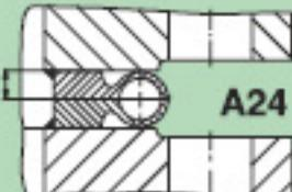
A24 | Standard procedure                                                                         | Not possible                                                                                       | Up to max. $\Delta r \sim 5$ mm depends on hollow lip wall thickness                       | Easy to dismantle with a 2mm cut off disc.<br>Can be re-welded up to 4 times         |
