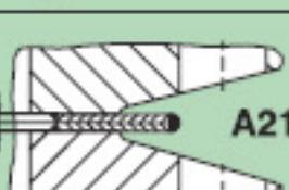
A21 | Only possible method                                                                       | Not possible.<br>Additionally flange form M to DIN 2526 required                                   | Effect is small and depends on projection of gaskets<br>max.. $\Delta r \sim 0,3$ mm       | Use cut-off disc.<br>Material loss 2-3 mm each.<br><br>Can be rewelded up to 5 times |
