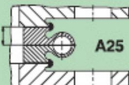
A25 | Can be applied as an additional intermittent weld for further fastening                    | Standard procedure                                                                                 | Up to max. $\Delta r \sim 5$ mm depends on hollow lip wall thickness                       | Easy to dismantle with a 2mm cut off disc.<br>Can be re-welded up to 4 times         |
