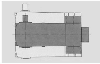
Comparison of spatial requirements for the new "T" configuration and standard parallel head type pump design.
