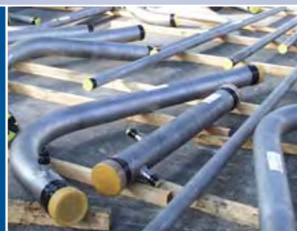
PREFABRICATED ISOMETRICS up to NS 10" 25Cr-22Ni-2Mo (BHDT A405)
