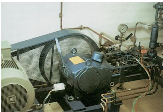
Figure 5 Liquid carbon dioxide pump with measuring instrumentation.
