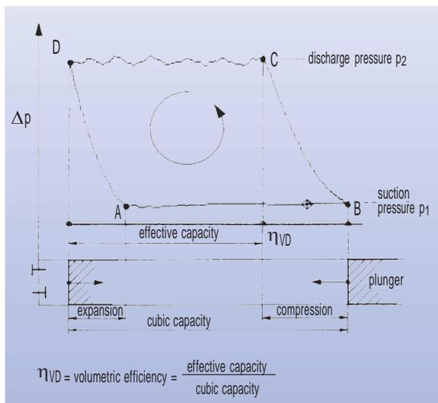
Figure 6 Indicator diagram for a reciprocating plunger pump in liquid carbon dioxide service.
