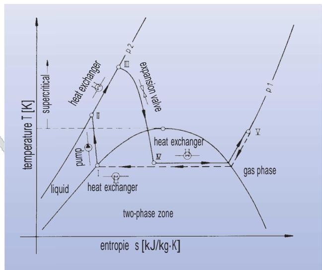
Figure 2 Temperature-Entropy Diagram (CO<sub>2</sub> Extraction Process).
