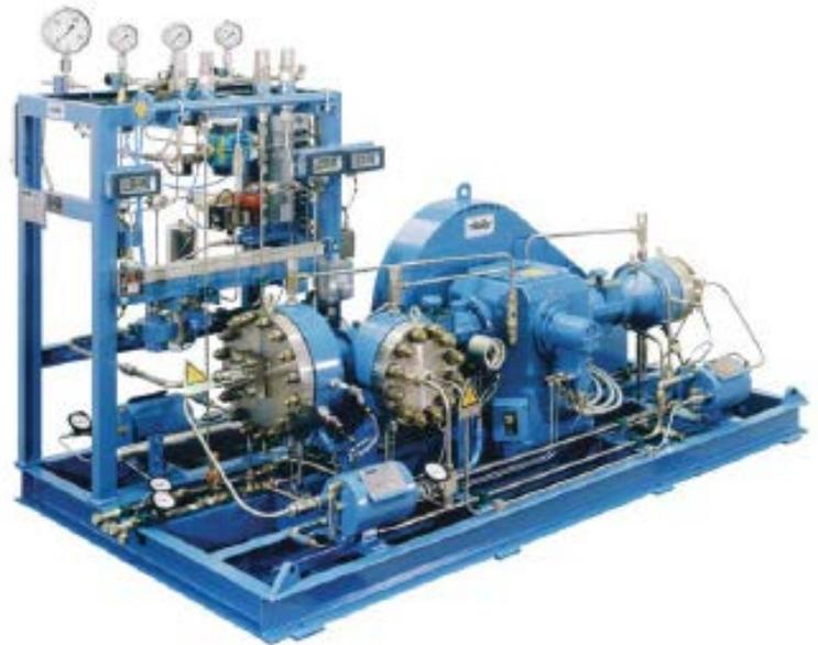
3-stage diaphragm compressor with digital oil-pressure indication display and oil-pressure supervision
