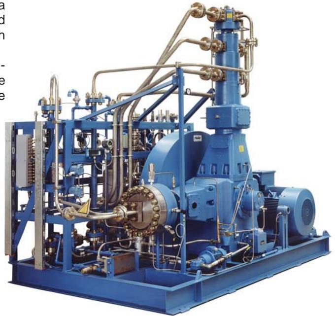
2-stage dry running piston compressor with final diaphragm stage
