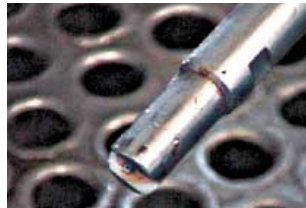
Top: Flexible and rigid lances. Bottom: Cleaning nozzle. The outlet openings of the cleaning jet can be seen at the front and the pushing nozzles can be seen at the side.
